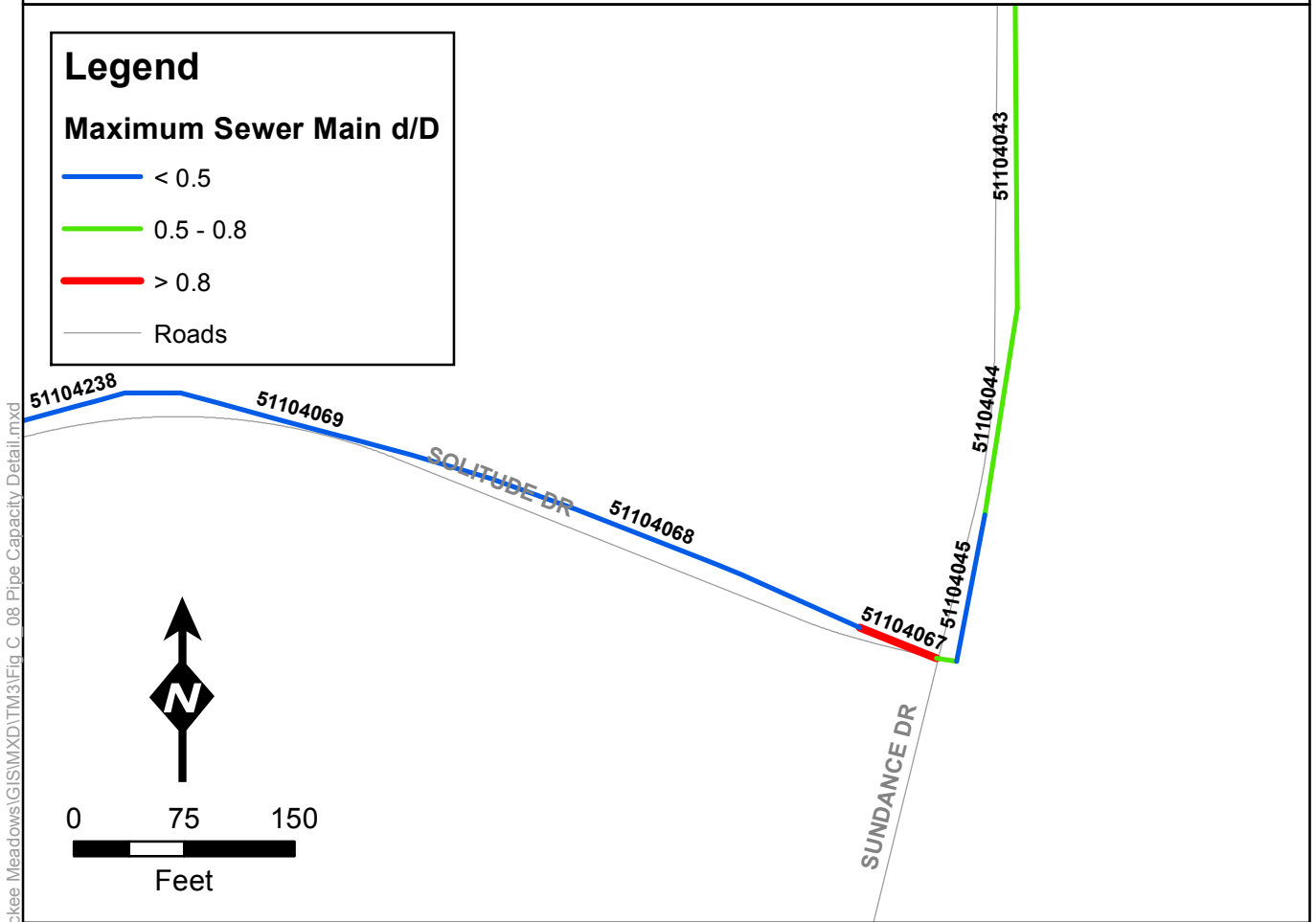
SEWER MAIN PLAN AND PROFILE WITH d/D NEAR SOLITUDE DR. AND SUNDANCE DR., BUILDOUT
